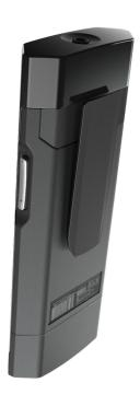
To increase the battery lifespan, the Lingua receiver is switched off when the headphone is disconnected. When signal reception becomes too low, the audio is muted. If the receiver does not receive any valid IR signal for more than 10 minutes, it automatically switches to standby.
