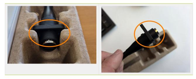
The following note explains how to remove and replace the plastic protector.
