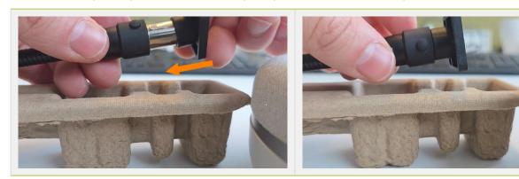
1 In case the microphones need to be stored and transported again in the packaging boxes, keep the protectors and replace them on the connectors when needed. If not, you can throw away the protectors.
