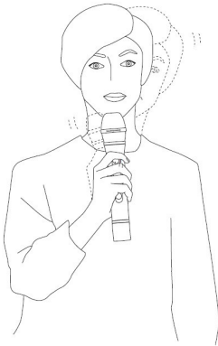
Figure 1-4 How to hold the microphone when using the "Near" setting
