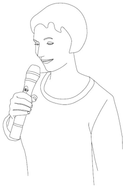
Figure 1-5 Optimum speaking distance when the ALC function is deactivated
