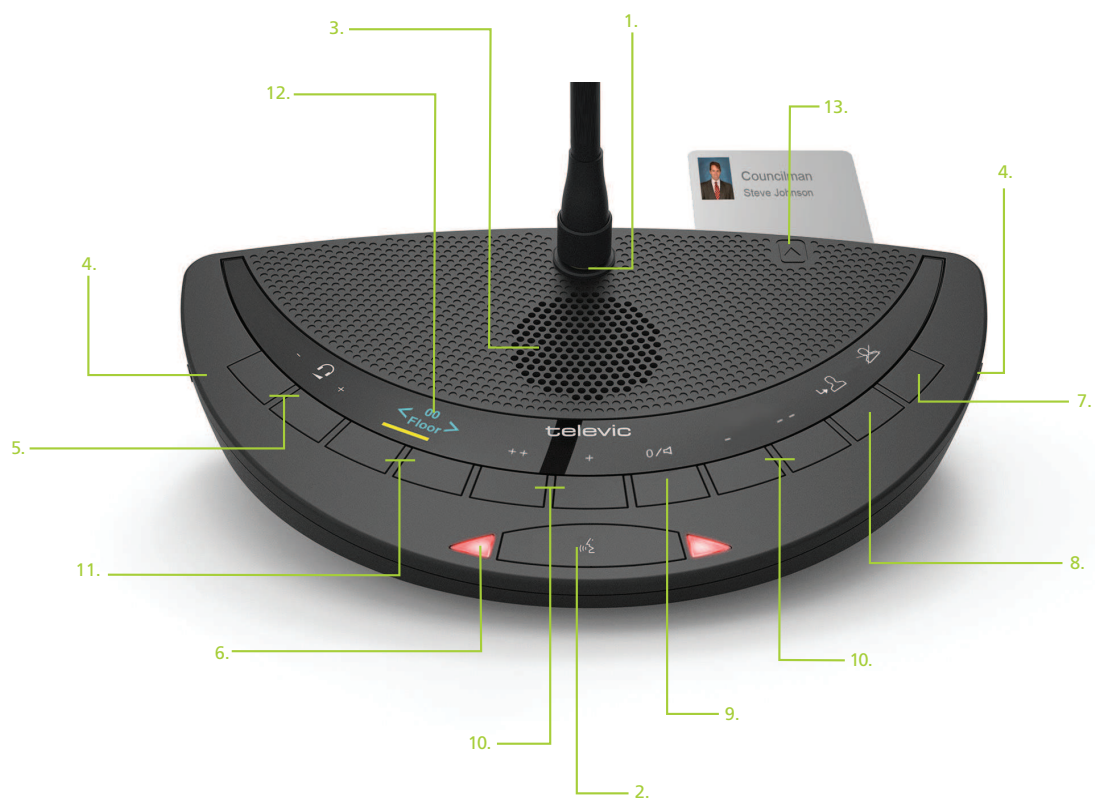
Figure 1-7 The front view of the Confidea G3 CIV unit with all possible options
