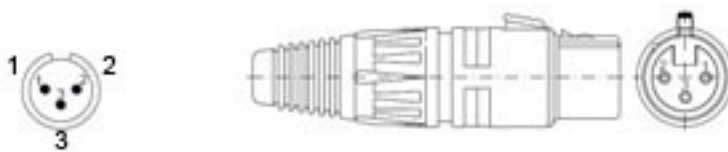
Figure 1-8 XLR pin assignment: Pin 1: Shield, Pin 2: Signal 2, Pin 3: Signal -
