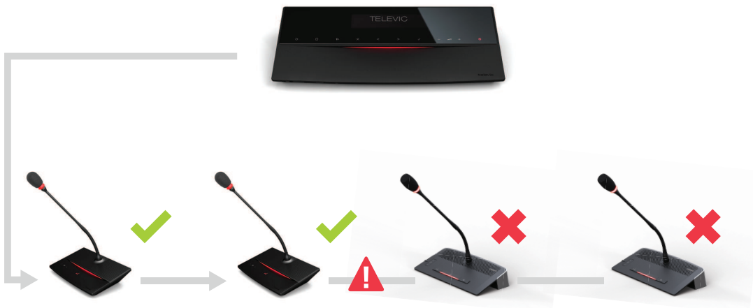
Figure 1-3 D-Cerno branch configuration with cable error, units after the cable are no longer active
