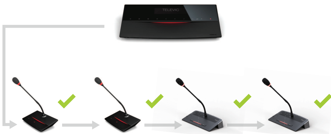
Figure 1-2 D-Cerno branch configuration, no error
