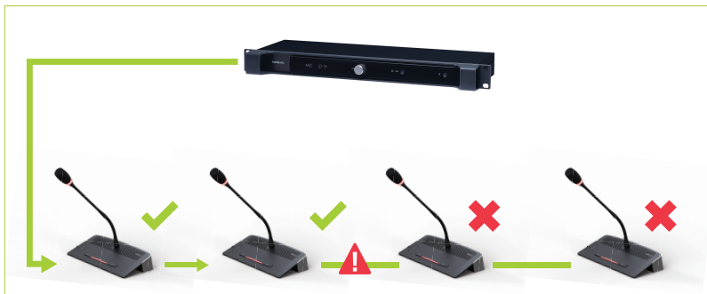
Figure 1-2 D-Cerno system branch configuration with cable error, units after the cable are no longer active
