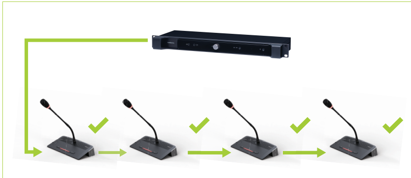
Figure 1-1 D-Cerno system branch configuration, no error
