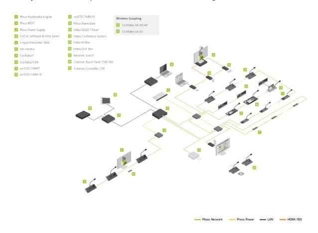
Both audio only and video enabled units can be integrated. These units can have a table top or flush mount form factor. Even combining wired and wireless units is supported.
