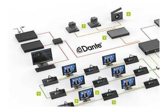
Audio can be routed over the AV network using the Dante or AES67 protocol. This gives a wide range of possibilities with Crestron DSP and amplifiers. Hybrid meetings with Teams, Zoom or Webex can easily be connected with the Crestron controlled room.
