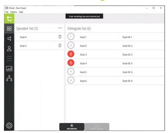
The Confero system can seamlessly be controlled using the certified Crestron integration. If allows to configure the microphone operation mode with the maximum open microphones, activate and deactivate microphones, volume control. Also voting and recording control is supported.
