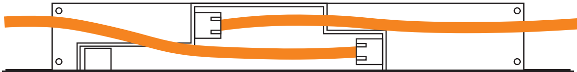
Figure 1-50 Bottom view of CAT 5e cabling of nameplate for portable usage
